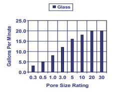
This chart represents typical water flow @ 1 PSID per 10" cartridge length. The test fluid is water at ambient temperature. Extrapolation for multiple elements tends to be linear, but as flows increase the DP of the housing becomes more apparent.
